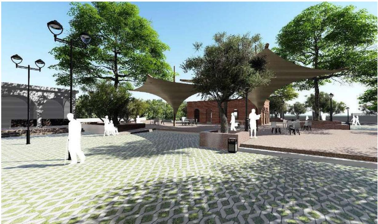
Figure 20: Tensile structures to provide shade to the outdoor sitting for heritage cafe. Note the seating provisions integrated with plantation beds, subtle level differences and floorscapes articulating different activity zones, and porous green-crete paving promoting sustainable environment
