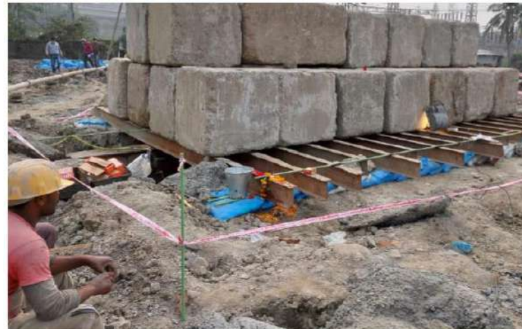
Vertical Load testing on pile at STP Near WBSETCL, Joka
