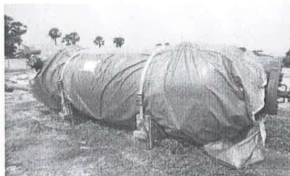
Proper storage of vessels- kept on saddles and lashed
