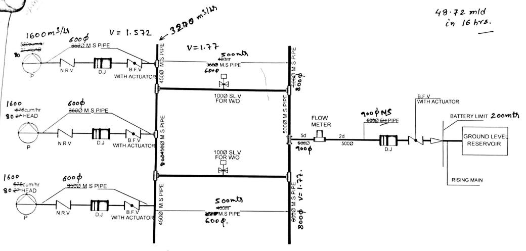
Pump duty: - 1600 m<sup>3</sup>/W H - 80 M.
