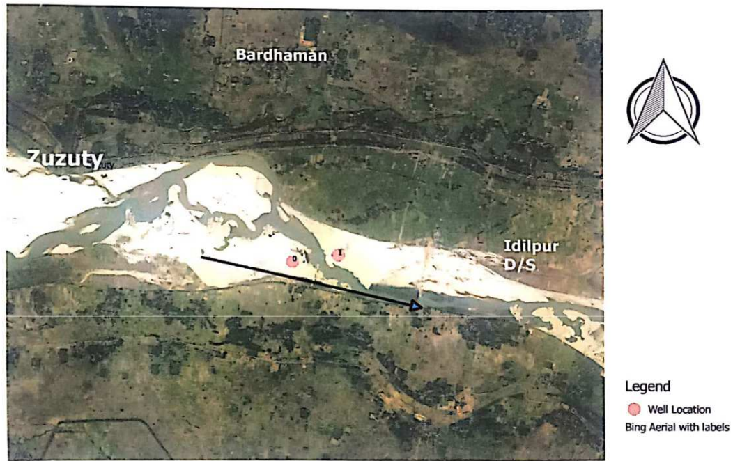
Figure 6.5: Recommended location for collector Well
