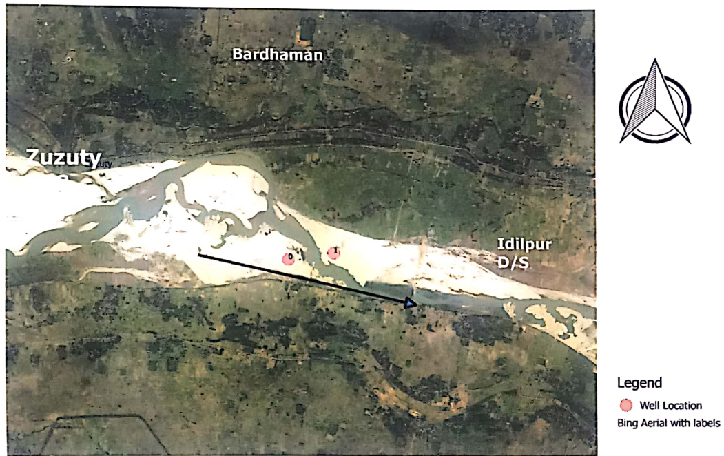
Figure 6.5: Recommended location for collector Well
